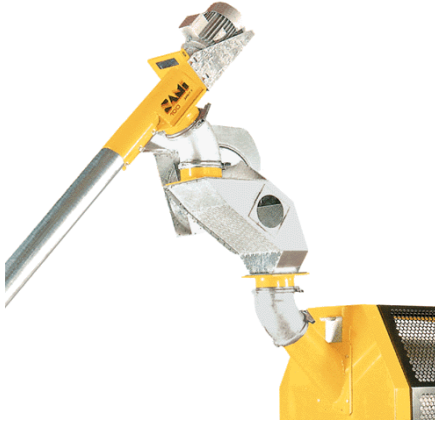
Figure 5. Screw conveyor and precleaner connected to the feeding tube
