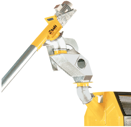
Figure 5. Screw conveyor and precleaner connected to the feeding tube
