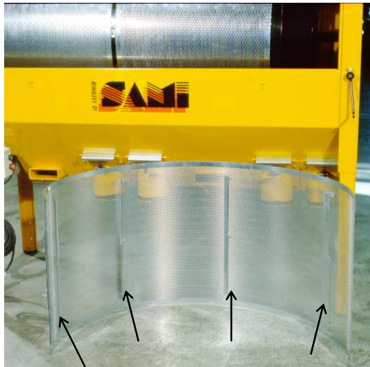
Figure 11. Attachment of mixing blades to the inner surface of a sieve
