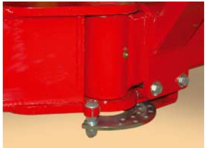
The body articulation brake is a standard accessory in Junkkari sprayers.
