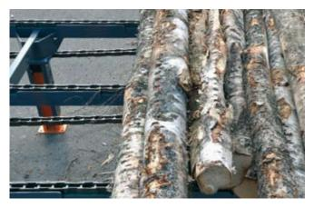
**1. TRANSFERRING WOOD ONTO THE LOADING TABLE** The wood is loaded onto the process-integrated loading table, which is equipped with chain conveyors.
