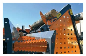
**5. TRANSFERRING LOGS INTO THE WAITING ROOM** After approved measuring, the bearers lift the log up and tip it through the restrainers in to the waiting room where the log waits for transfer conveyor to be available again.
