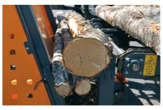
**2. FEEDING WOOD TO THE SORTER** The sensors of the sorter frame activate the loading table to feed wood to the sorter. The loading table conveys wood onto the sorter's table, against the sorter's frame.
