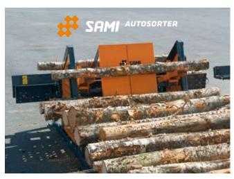
**AT WIDEST, SAMI AUTOSORTER** consists of a loading table, a sorter and a transfer conveyor. SAMI Autosorter integrated in SAMI Autochopper – the entire log splitting process is automatic.
