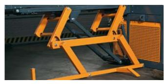
**THE HYDRAULIC LOG LIFTER** minimizes physical work phases and is safe to use because of its completely vertical lifting direction. Attached to the feed table, it does not lean against the ground, which makes it easily movable with the feed table. Consequently, the lifter is also always read for use.
