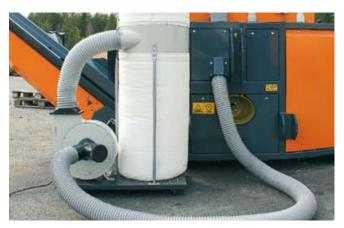
**THE SAWDUST EXTRACTOR** traps all sawdust neatly into a container. A compact model runs on mains electricity, the larger exhauster on 3-phase power.
