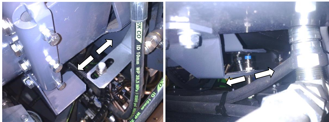
Figure 38. Adjusting the stroke length of the splitting
