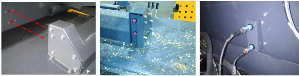
Figure 28. The optical sensors of the feed conveyor
