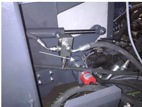
Figure 57 Bearing of axe lever, 1 grease nipple
