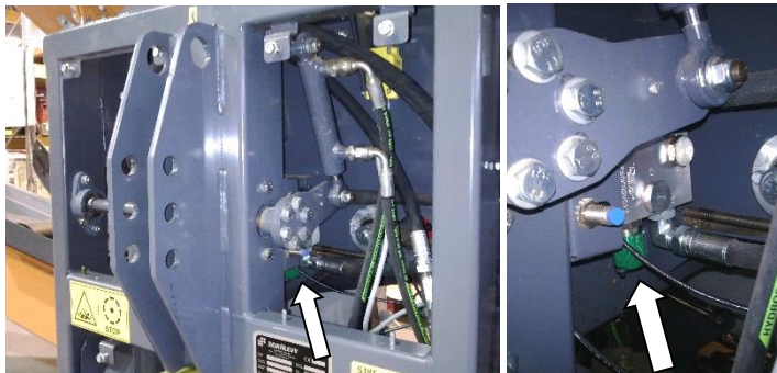
Figure 37. Adjusting the speed of the feed belt
