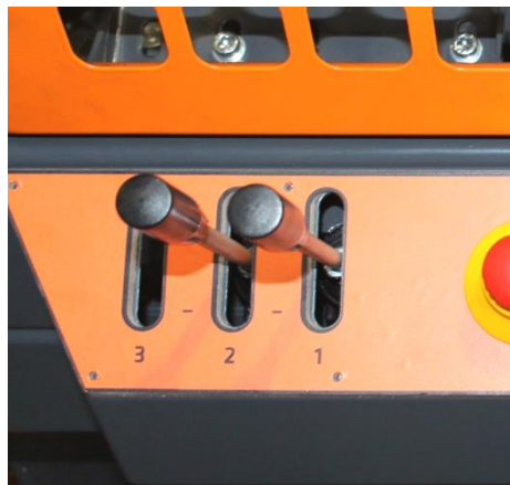
Figure 6 Hydraulic levers: 1. Position of discharge conveyor; 2. Position of hydraulic log lifter (accessory) and feed conveyor; “+” = conveyor up; “-” = conveyor down.
