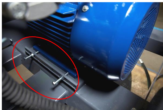
Figure 53 Tightening of V-belt from the base of the electric motor
