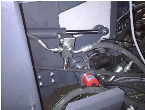
Figure 31. The angle sensor of the splitting blade
