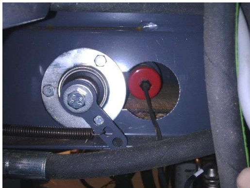
Figure 29. The angle sensor of the feed belt
