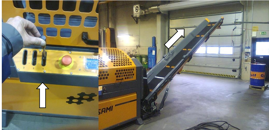
Figure 10. Using the telescope of the discharge conveyor
