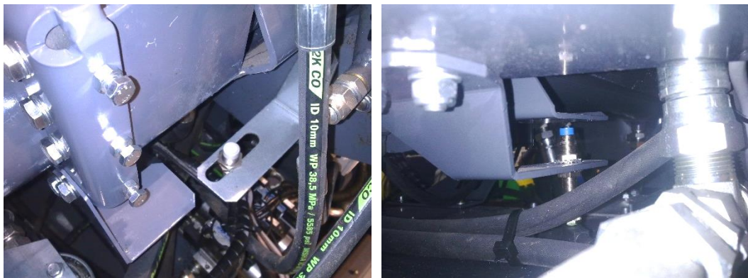
Figure 33. The inductive front and rear sensors of the splitting cylinder
