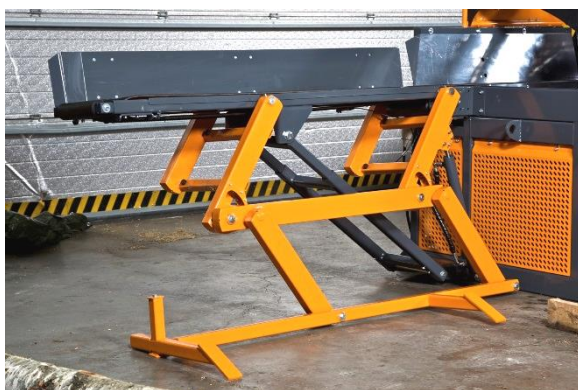
Figure 54 Log lifter, 12 grease nipples (accessory)
