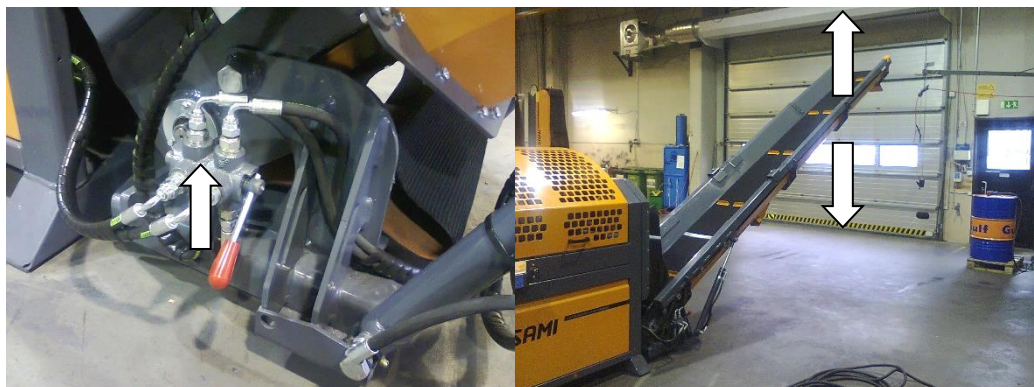
Figure 11. Adjusting the height of the discharge conveyor
