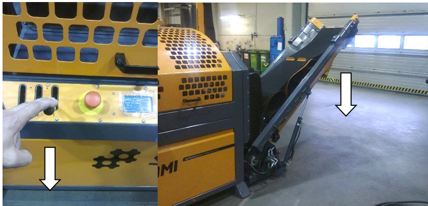
Figure 8. Lowering the discharge conveyor
