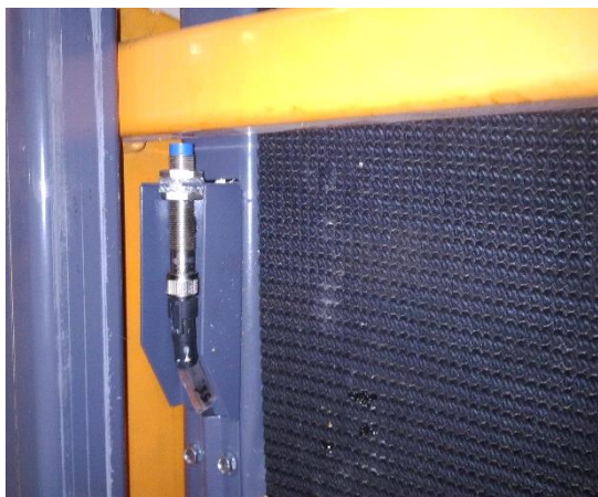
Figure 34. The inductive sensor of the log lifter
