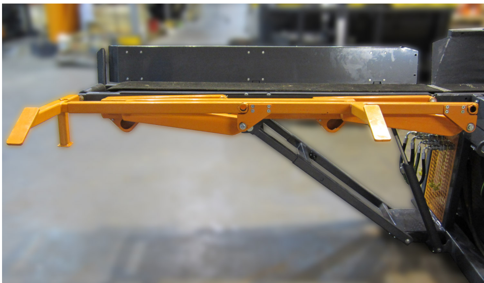
Log lifter flush with the feed conveyor.
